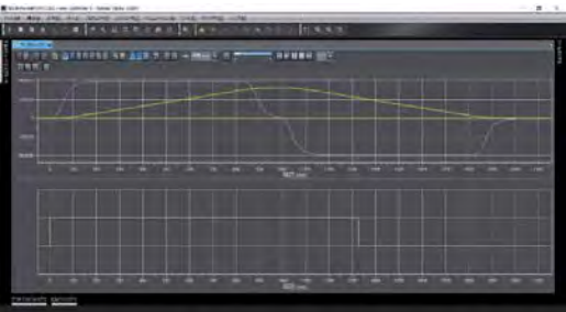
Example) Monitoring of position, velocity and electric current value by SysmacStudio (made by OMRON).
