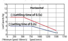
Graph (1) is for standard specifications, with settling time of 0.5s for calculating the positioning time. Graph② reflects some changes in the controller settings. The load capacity is lower, however the settling time is decreased to 0.2s.
