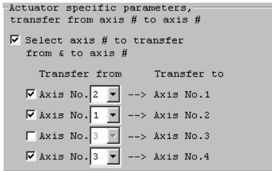
In the specification example shown to the left, data for axis 2 in the file is sent to axis 1 in the controller, data for axis 1 in the file is sent to axis 2 in the controller, and data for axis 3 in the file is sent to axis 4 in the controller, respectively. (No data will be sent to axis 3 in the controller.)
