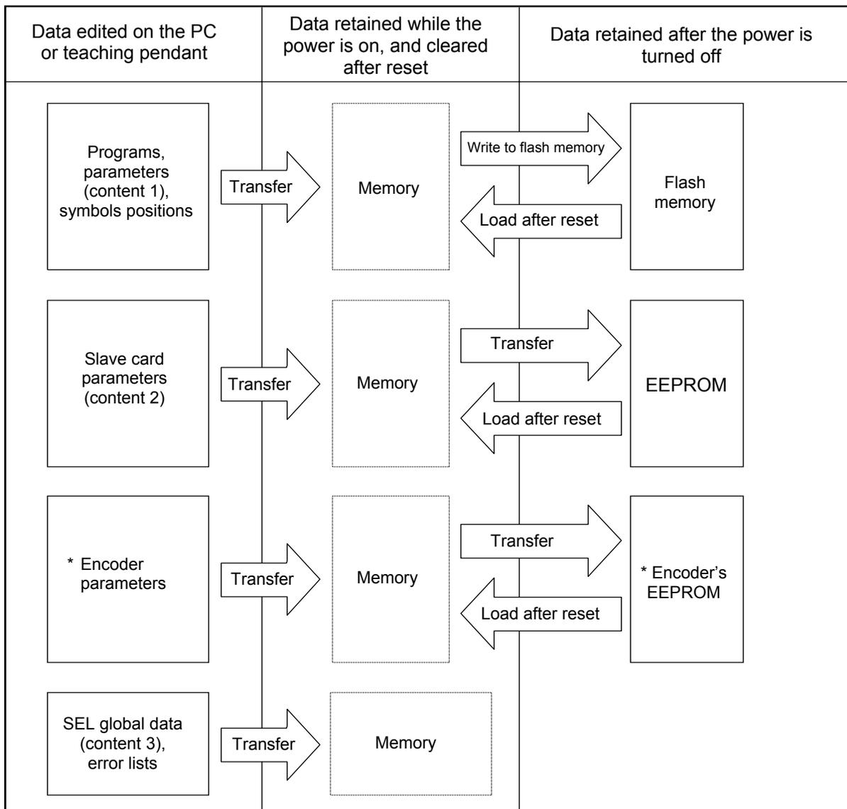
Programs, parameters and symbols are loaded from the flash memory after a restart. Unless written to the flash memory, therefore, edited programs, parameters and symbols will return to the original data once the controller is restarted.
