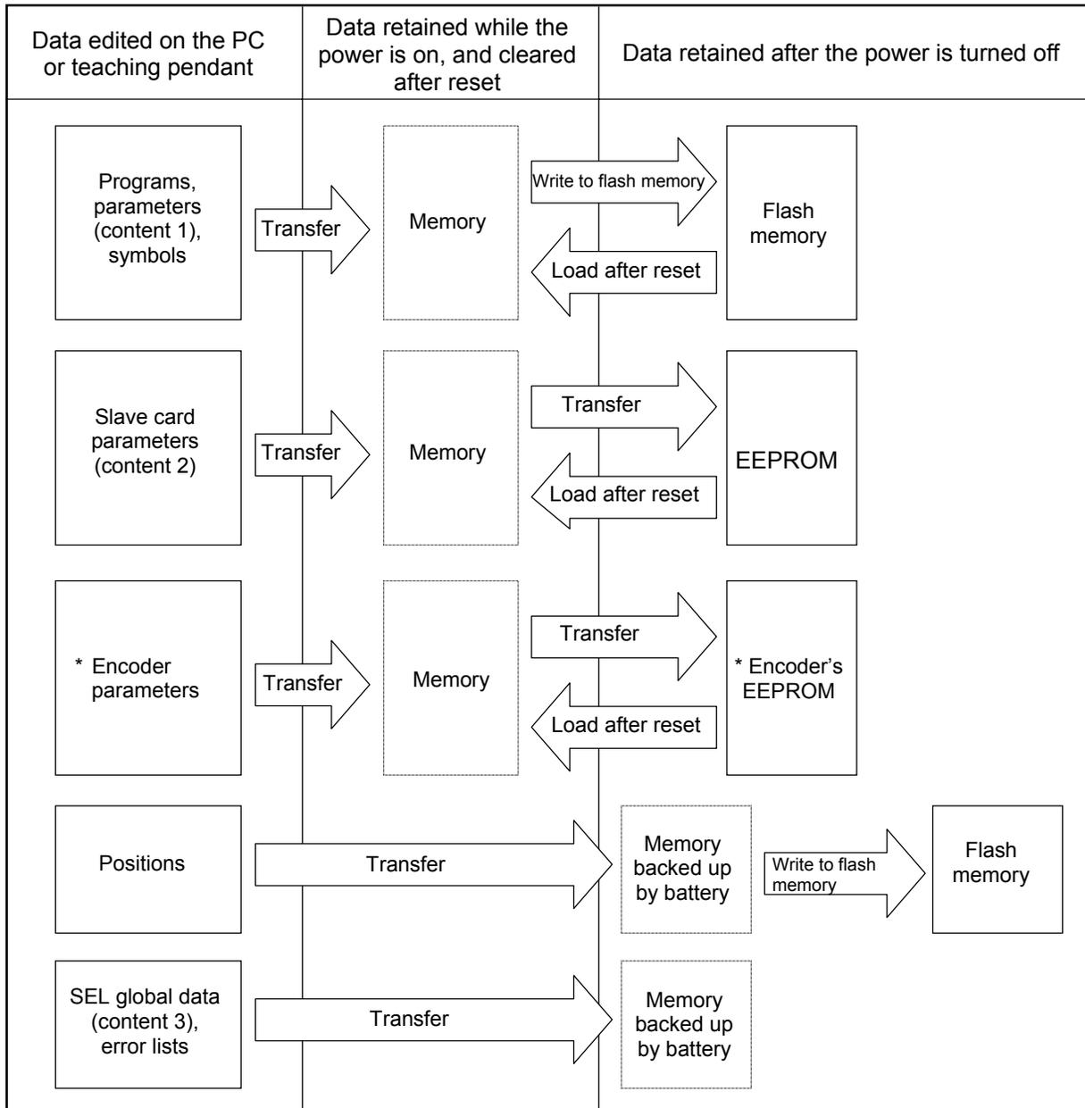
\* Encoder parameters are stored in the EEPROM of the actuator's encoder, not in the controller's EEPROM. Therefore, encoder parameters will be loaded to the controller every time the controller power is turned on or a software reset is executed.
