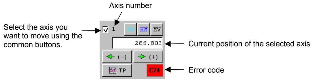
Fig. 6.4 Axis-specific buttons
