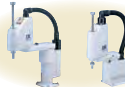
Synchronous control of two SCARA robots
