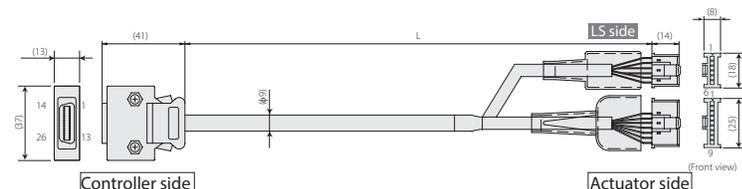
Minimum bending radius  $r = 54\text{mm}$  or more (Dynamic bending condition)
