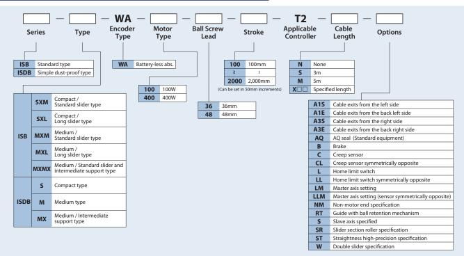
\*The type of motor, ball screw lead, stroke, and options vary depending on the actuator type. Please refer to the reference page of each type for details.
