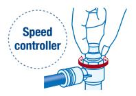
Transfer time cannot be accurately shown because the speed controller is analog. In addition, the cycle time changes largely depending on the operating environment, season, temperature and aged deterioration of packings.
