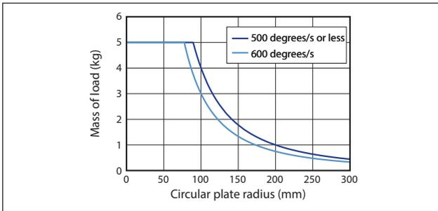
When the center of gravity of the load is offset from the rotational center of the output shaft
