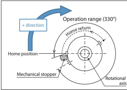
The positive rotation direction will be clockwise when viewing the rotating part from above. During home return motion, it rotates counterclockwise. It detects the mechanical stopper position, moves in reverse, and then stops. It cannot rotate to the home return motion in the clockwise direction. (Note) For the non-motor end specification, all movement directions are in reverse.
