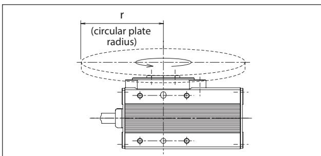
■ When the center of gravity of the load is offset from the rotational center of the output shaft
