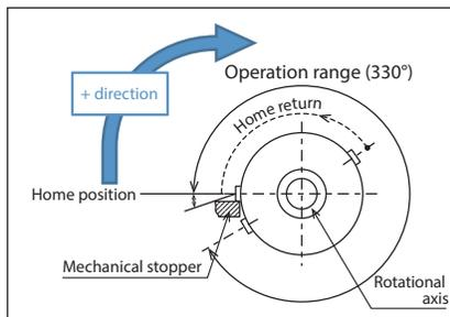
The positive rotation direction will be clockwise when viewing the rotating part from above.
