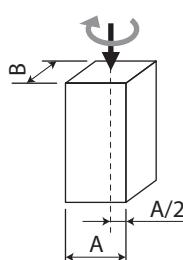
**2. When the center of the object is offset from the rotational axis****(4) Moment of inertia of cylinder 3**
