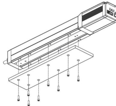
● Using the front bracket screw hole
