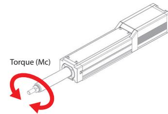
2. The torque (Mc) acting on the rod must not exceed the allowable value.
