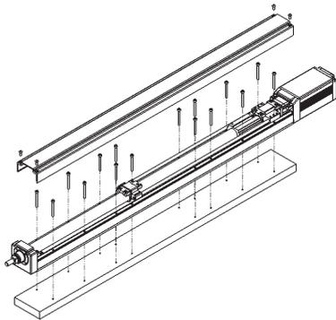
● Using the base bottom surface screw hole
