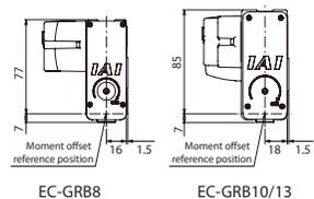
Even with the grip point distance within the limit range, keep the finger attachment as small and lightweight as possible.
