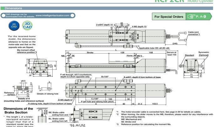
\* The length L of a brake-equipped actuator is longer than that of a standard model (see the table) by 43mm (56.3mm with the cable exit out its end); add 0.6kg to weight.
