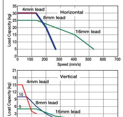
Actuator Specifications ■ Lead and Load Capacity
