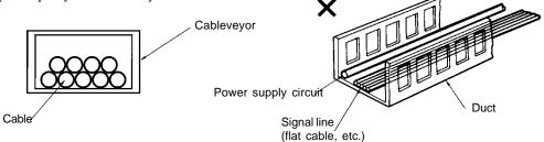
10 In a case where the cable will be subject to forced bending, always use robot cable.
