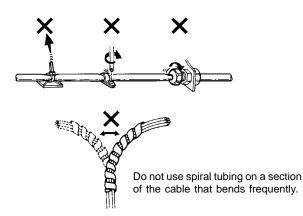
7 If placing cable in a cableveyor or flexible tube, make sure it does not twist around. Also, make sure the cables have some freedom of movement and are not bunched up (cable should not project out at bending points).
