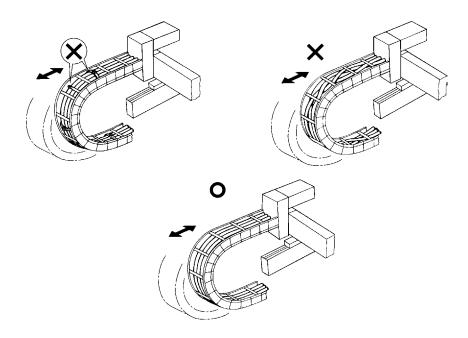
**8** The amount of cable placed inside a cableveyor should be about 60% of the space capacity of the cableveyor.
