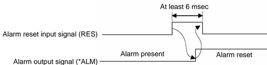
⚠ Caution: Before resetting an alarm, always identify and remove the cause of the alarm. If the cause cannot be removed or the alarm still persists after removing the cause, contact IAI. If the same error occurs again after resetting the alarm, the problem that caused the alarm in the first place is still present.
