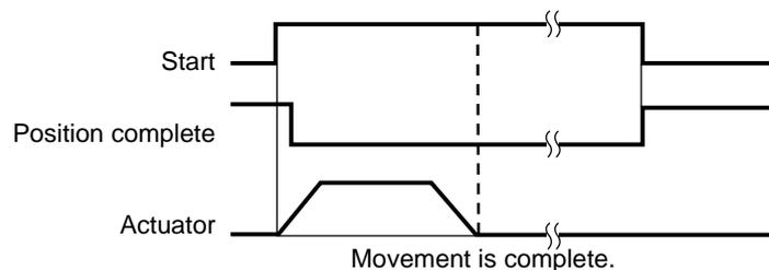
The diagram shows a scenario where the Start signal is turned ON and remains ON. The Actuator signal shows a trapezoidal movement that is completed. However, because the Start signal is still ON, the Position complete signal does not turn ON. A vertical dashed line indicates the point where 'Movement is complete'.
