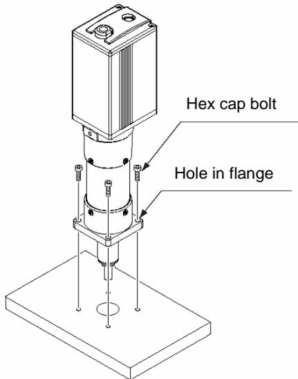
**⚠ Caution:** If the actuator is installed horizontally, exercise caution not to let the actuator receive excessive forces.
