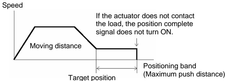
(3) Load moves during push & hold operation
