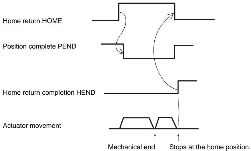
**⚠ Caution:** When the home return signal turns ON, the position complete output will turn OFF. Always turn OFF the home return signal after confirming that the home return completion output has turned ON.
