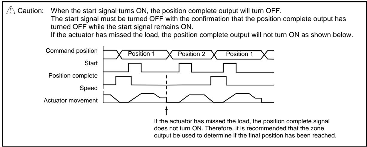
If the actuator has missed the load, the position complete signal does not turn ON. Therefore, it is recommended that the zone output be used to determine if the final position has been reached.
