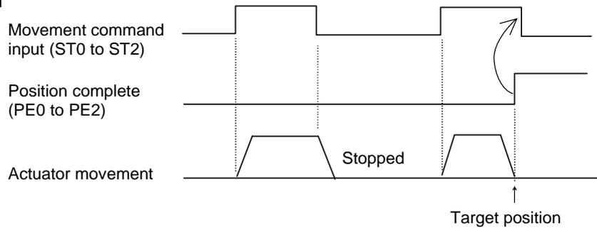
(Note) Turn OFF the movement command input after confirming that the target position has been reached.
