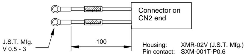
(Note) Connecting 24V to the SGA/SGB serial-communication lines will cause a breakdown. To prevent miswiring, a two-pin connector is installed at the ends of the applicable lines. If multiple axes are linked, connect these supplied cables to the CN2 connector and extend as required, or cut them off at the base of the CN2 connector and install crimp terminals directly.
