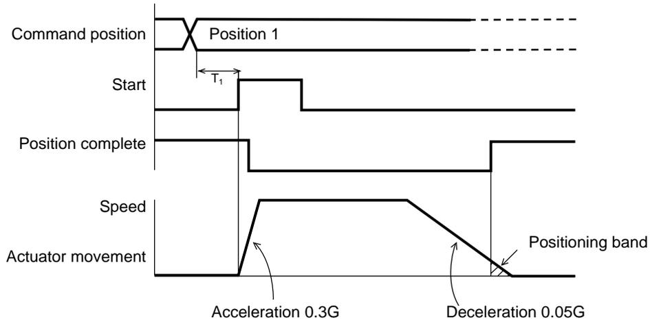
T1: 6 msec or more; time after selecting/entering a command position until the start input turns ON (The scan time of the host controller must be considered.)
