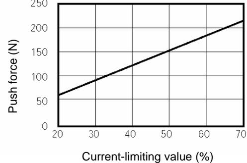
⚠ Caution: The accuracy of push force at standstill is not guaranteed. The above graphs are provided for reference purposes only. If the push force is too small, malfunction may occur during push & hold operation due to slide resistance, etc., so exercise caution. The maximum current-limiting value is shown in the above graphs. The minimum value is 20%.
