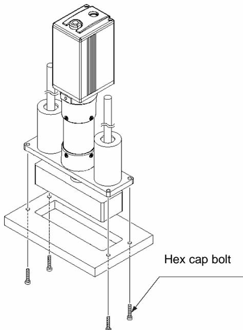
**⚠ Caution:** If the actuator is installed horizontally, exercise caution not to let the actuator receive excessive forces.
