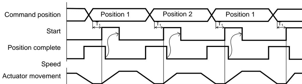
T1: 6 msec or more; time after selecting/entering a command position until the start input turns ON
