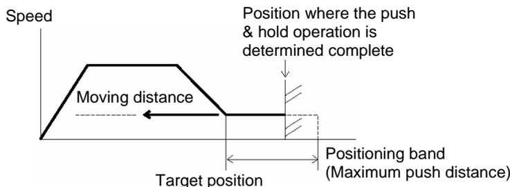
(Note) If the actuator is pushed back to the target position, an alarm will occur.
