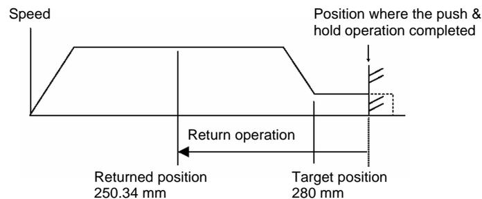
**⚠ Caution:** When the start signal turns ON, the position complete output will turn OFF. The start signal must be turned OFF with the confirmation that the position complete output has turned OFF while the start signal remains ON. If the actuator has missed the load, the position complete output will not turn ON as shown below.
