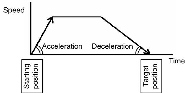
Increasing the set value makes acceleration/deceleration quicker, while decreasing the set value makes acceleration/deceleration more gradual.
