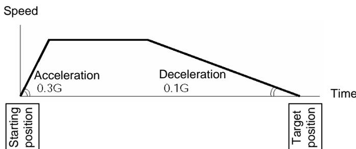
⚠ Caution: Basically, you should set the acceleration/deceleration within the rated range specified in the catalog. The input range is greater than the rated range in the catalog, in order to accommodate situations where you want to "shorten the tact time when the load is much smaller than the rated load capacity." If the actuator is to be operated in this condition, however, its service life may be affected. Contact IAI beforehand for consultation.
