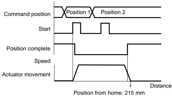
If the start signal for movement to an incremental position number is input multiple times during positioning, the actuator will move to the position corresponding to the initial position plus the "increment x number of times the signal was input."
