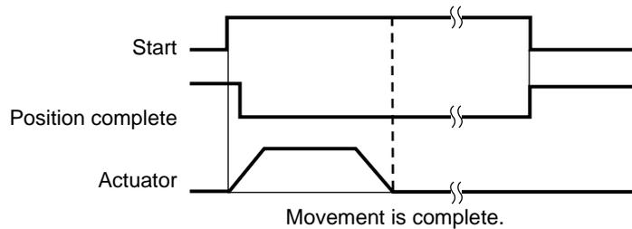
Note 2: When a soft limit is reached as a result of repeated incremental moves, the actuator will stop at that position and the position complete signal will be output.
