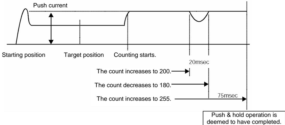
If the motor current remains at or above the push current for 200 msec and then drops below this level for 20 msec, the count will decrease by 20. When the push current is reached again thereafter, counting will start from 180. If the motor current remains at or above the push current for 75 msec, the count will increase to 255 and thus push & hold operation will be deemed to have completed.
