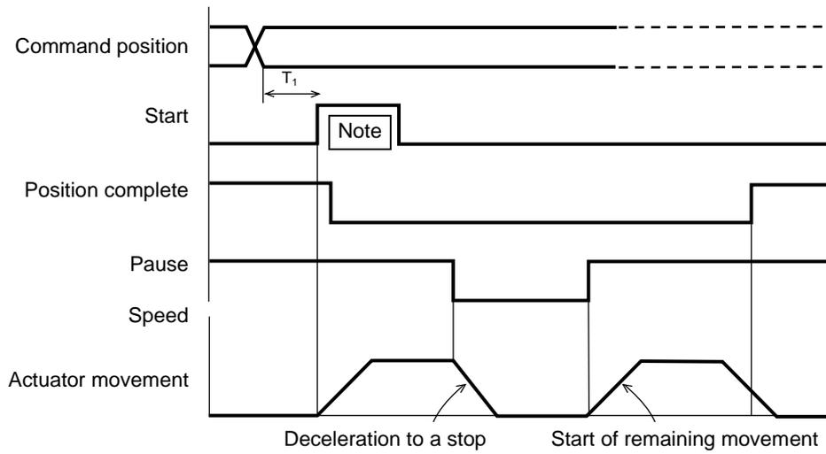
T1: 6 msec or more; time after selecting/entering a command position until the start input turns ON
