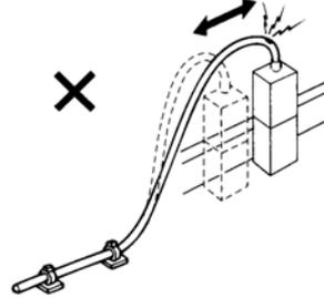
4. Do not let the cable receive a turning force at a single point. 5. When fixing the cable, provide a moderate slack and do not tension it too tight.
