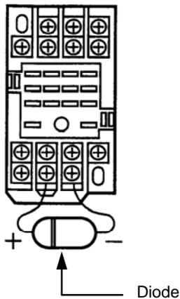
In a DC circuit, connecting a diode in reverse polarity will damage the diode, internal parts of the controller and/or DC power supply, so exercise due caution.
