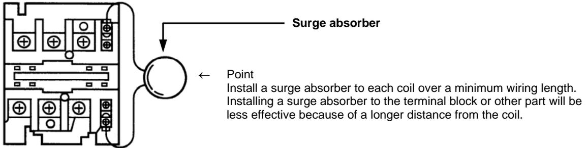
[2] DC solenoid valves, magnet switches and relays
