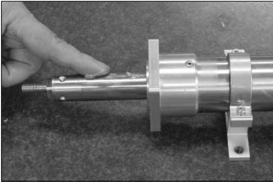
**!** Note: Never use fluorine grease. If fluorine grease is mixed with lithium grease, the grease function will drop and it causes damage to the mechanism.
