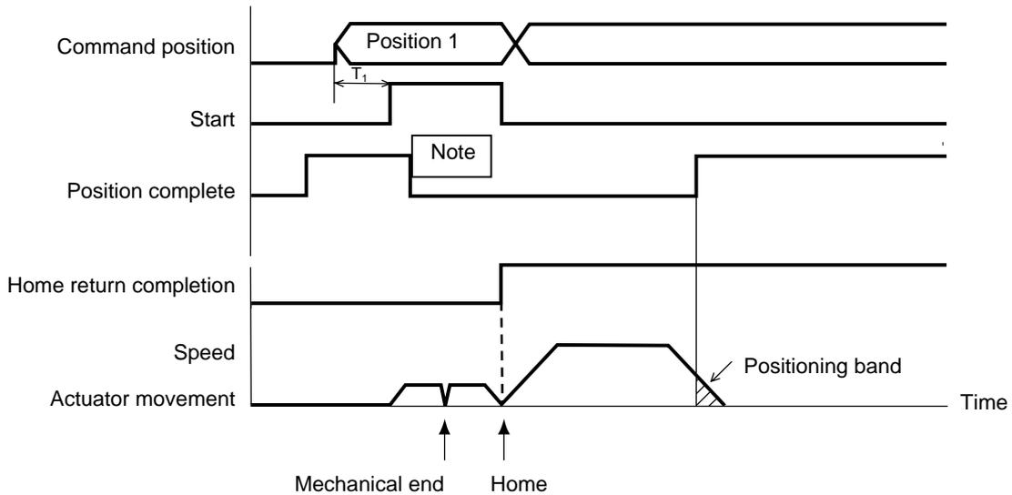
The position complete output will turn ON when the controller becomes ready following the power ON. To check if the controller is ready, always check if the position complete output is ON.
