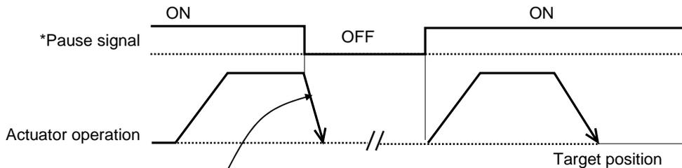
(Note) The deceleration becomes the value set in the "Deceleration" field of the position table for the position number corresponding to the current positioning operation.
