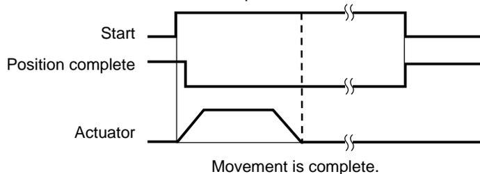
[2] Increasing the positioning band allows the position complete signal to turn ON more quickly, and consequently the next operation in the sequence starts early. This is an effective means for reducing the tact time, so set an optimal value based on the overall balance of your system.
