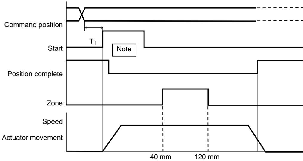
T1: 6 msec or more; time after selecting/entering a command position until the start input turns ON (The scan time of the host controller must be considered.)
