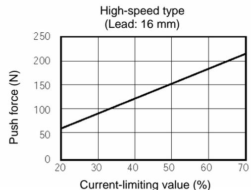
⚠ Caution: The accuracy of push force at standstill is not guaranteed. The above graphs are provided for reference purposes only. If the push force is too small, malfunction may occur during push & hold operation due to slide resistance, etc., so exercise caution. The maximum current-limiting value is shown in the above graphs. The minimum value is 20%.
