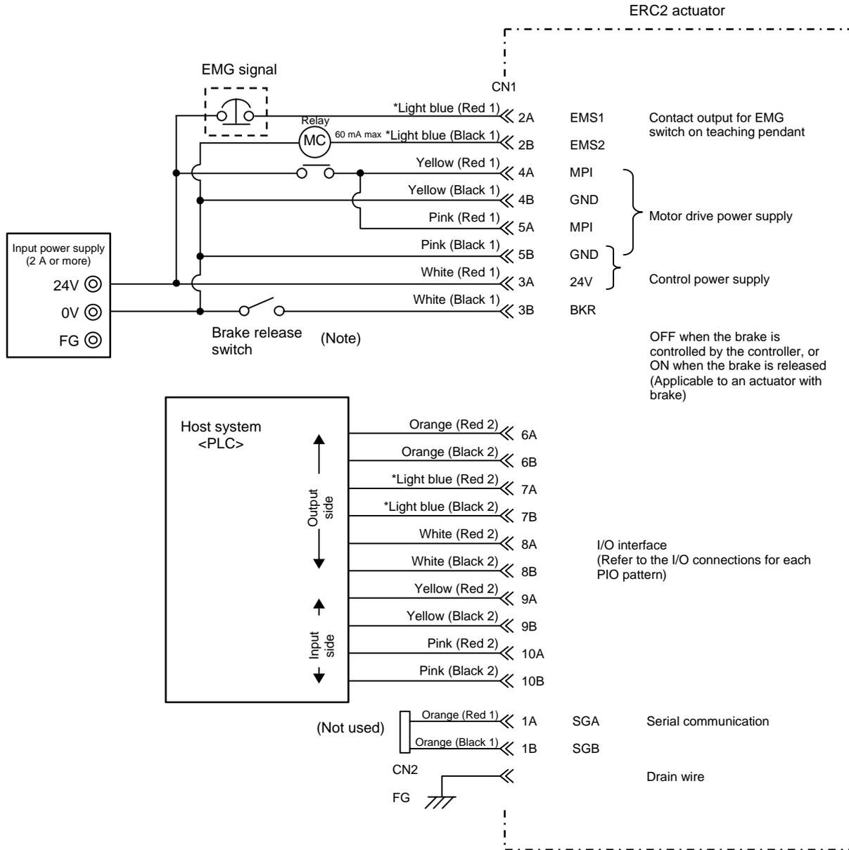
\* In the case of a robot cable, the wire colors change as follows.
