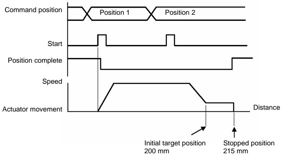
● Moving in the push & hold mode to the position number set in the incremental mode
