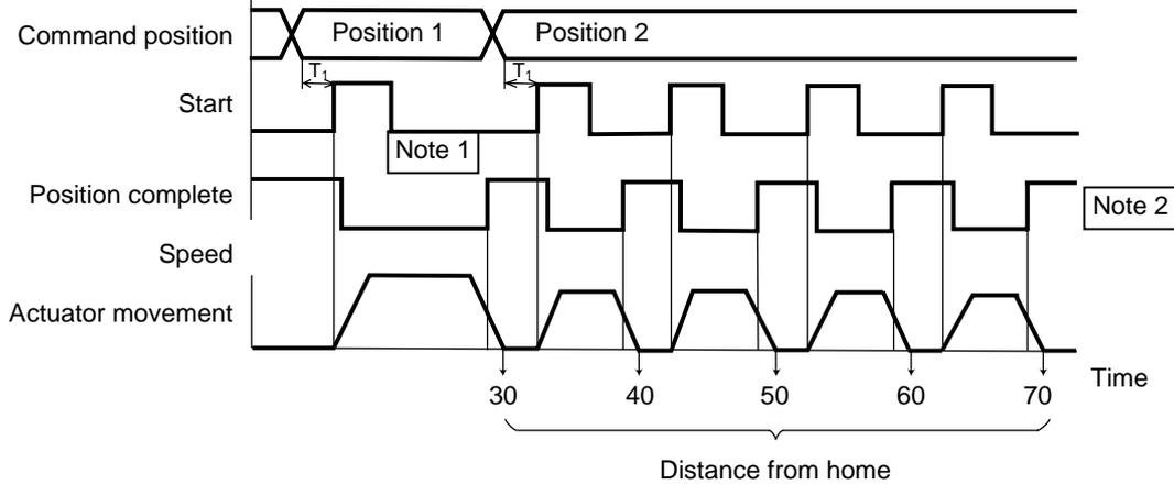
T1: 6 msec or more; time after selecting/entering a command position until the start input turns ON (The scan time of the host controller must be considered.)
