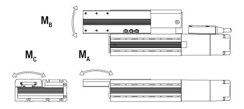
The points of moment application in the Ma and Mb directions are as shown below.
