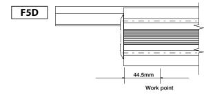
Be careful that the load exerted on the plate tip does not exceed the Ma moment when using a flat type horizontally.
