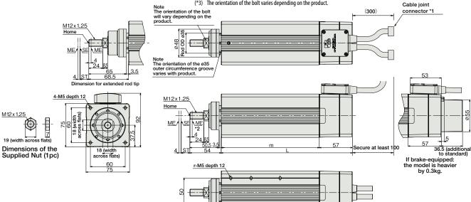
Note: Do not apply any external force on the rod from any direction other than the direction of the rod's motion. If a force is exerted on the rod in a perpendicular or rotational direction, the detent may become
