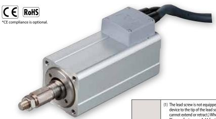
(1) The lead screw is not equipped with an anti-rotation device, so please attach a guide or similar locking device to the tip of the lead screw prior to use. (If there is no anti-rotation device attached, the lead screw cannot extend or retract.) When connecting the anti-rotation device and rod, do not use a floating joint. Please refer to page A-11 for the instruction details.
