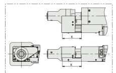
Length of a cable track cover only for up to 270mm-stroke
